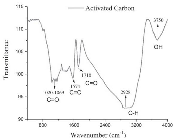
Fig. 2. FTIR spectra of ATNPP sample
